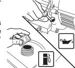
Never fill fuel tank completely. Fill tank to 1/2" below the bottom of the filler neck to provide space for fuel expansion. Wipe any fuel spillage from engine and equipment before starting engine.
